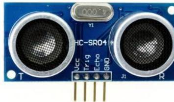
*Figure 3 Ultrasonic Sensor*
