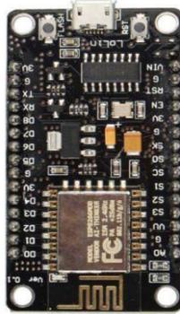
Figure 4 NODEMCU DEV 1.0 ESP8266
